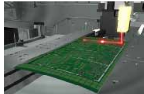
Figure 5: Board Mapping Concept in a Pick and Place Machine
