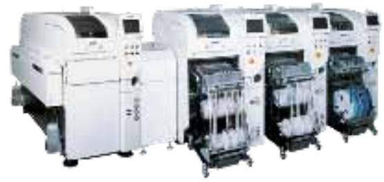
Figure 4: Panasonic NPM-DSP Printer with NPM-D2 Pick and Place Used during Test Builds
