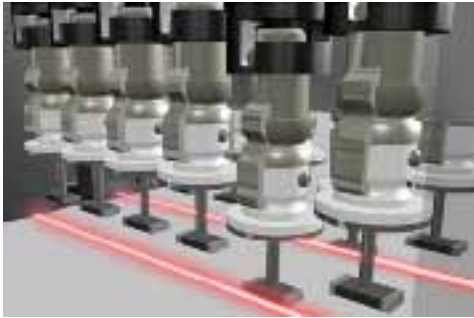
Figure 6: Head-mounted Side View Camera Concept in a Pick and Place Machine
